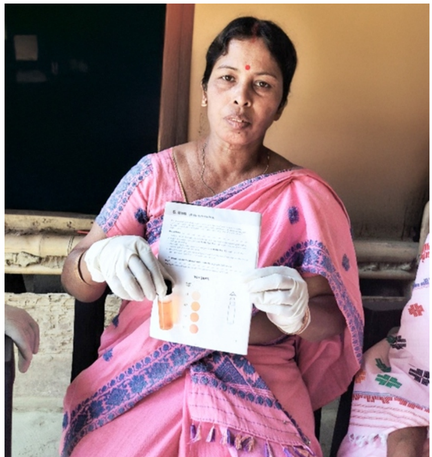
Figure 29: Dalimi Rajbongshi displays the iron test results, referencing the chart for accurate interpretation | Source: CML Tata Trusts
