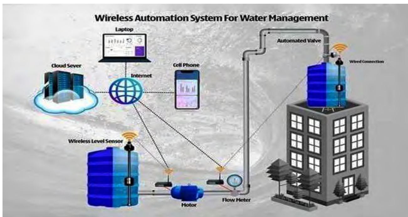
Figure 19: The Wireless Automation System of Water Management | Source: Water Supply and Sanitation Department, Maharashtra
