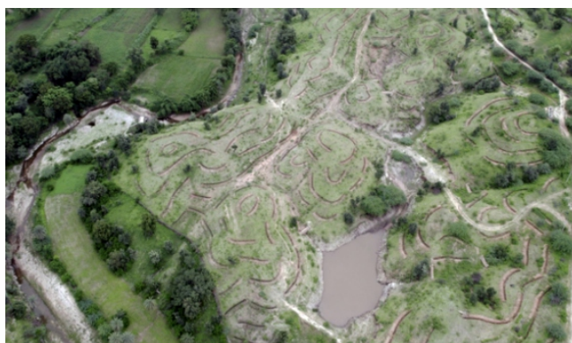
Figure 14-15: Targeting Source sustainability of drinking water source created under Jal Jeevan Mission (JJM), Water recharge and harvesting works were executed adopting ridge to valley approach in Bothara village | Source: CmF Tata Trusts
