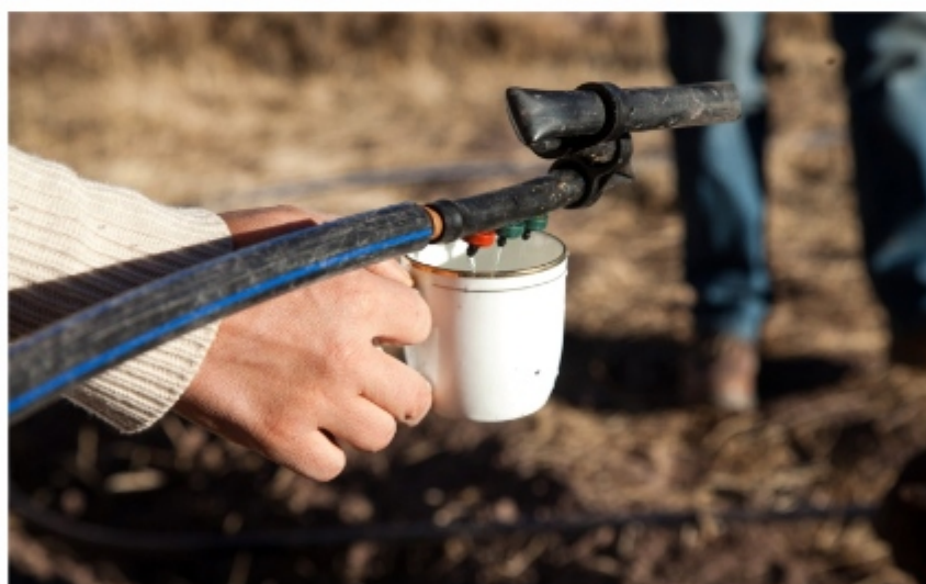
Figure 65: The colour-coded dripper mechanism | Source: PHE Leh
