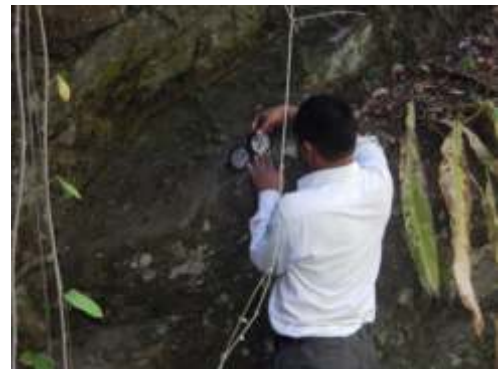
Photo 5: Hydrogeological Survey through Brunton
